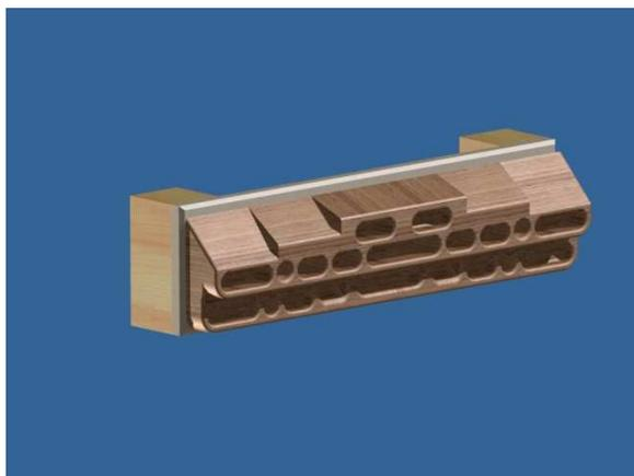
This shows the fingerboard mounted on a piece of plywood which is attached to the wall via 2 blocks of wood. The blocks provide clearance under the fingerboard – so it sticks out beyond the doorframe allowing your fingers to hang freely off holds and not grind on the door frame. It also provides clearance for screws which attach the fingerboard to the plywood – preventing them from damaging the wall behind.
